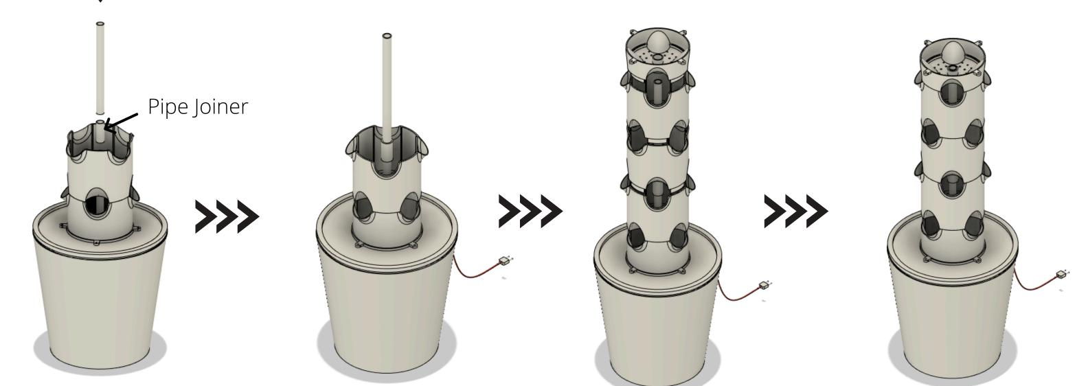
Connect another piece of pipe with pipe joiner
